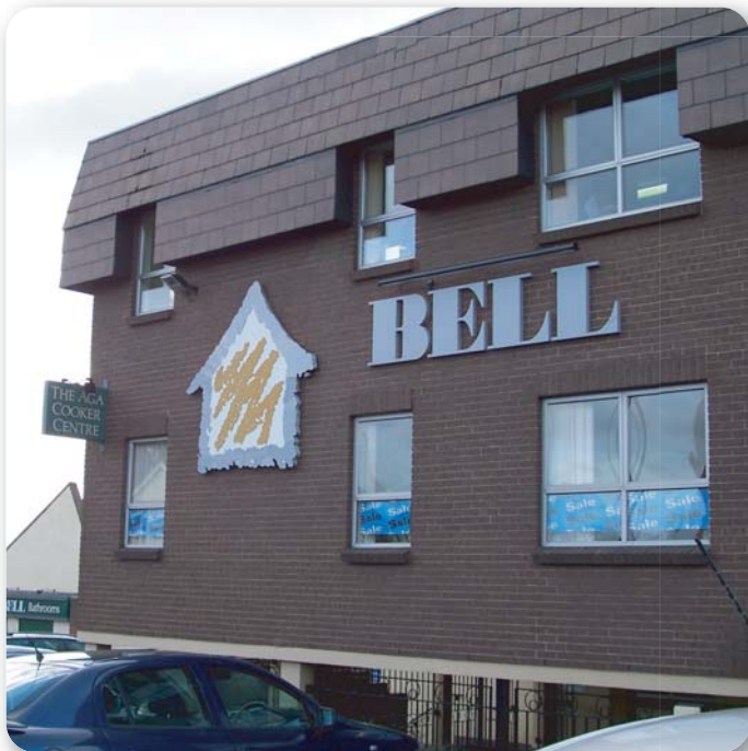
Built-up letters and logo externally illuminated with a trough light
