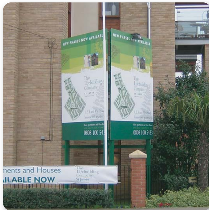
Laminated wide format digital prints applied to aluminium post sign
